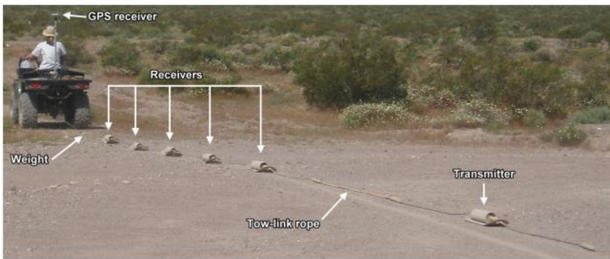
Figure 2-1. The OhmMapper system shown with five receiver dipoles and the transmitter dipole towed by an all-terrain vehicle (Lucius et al. 2008)
