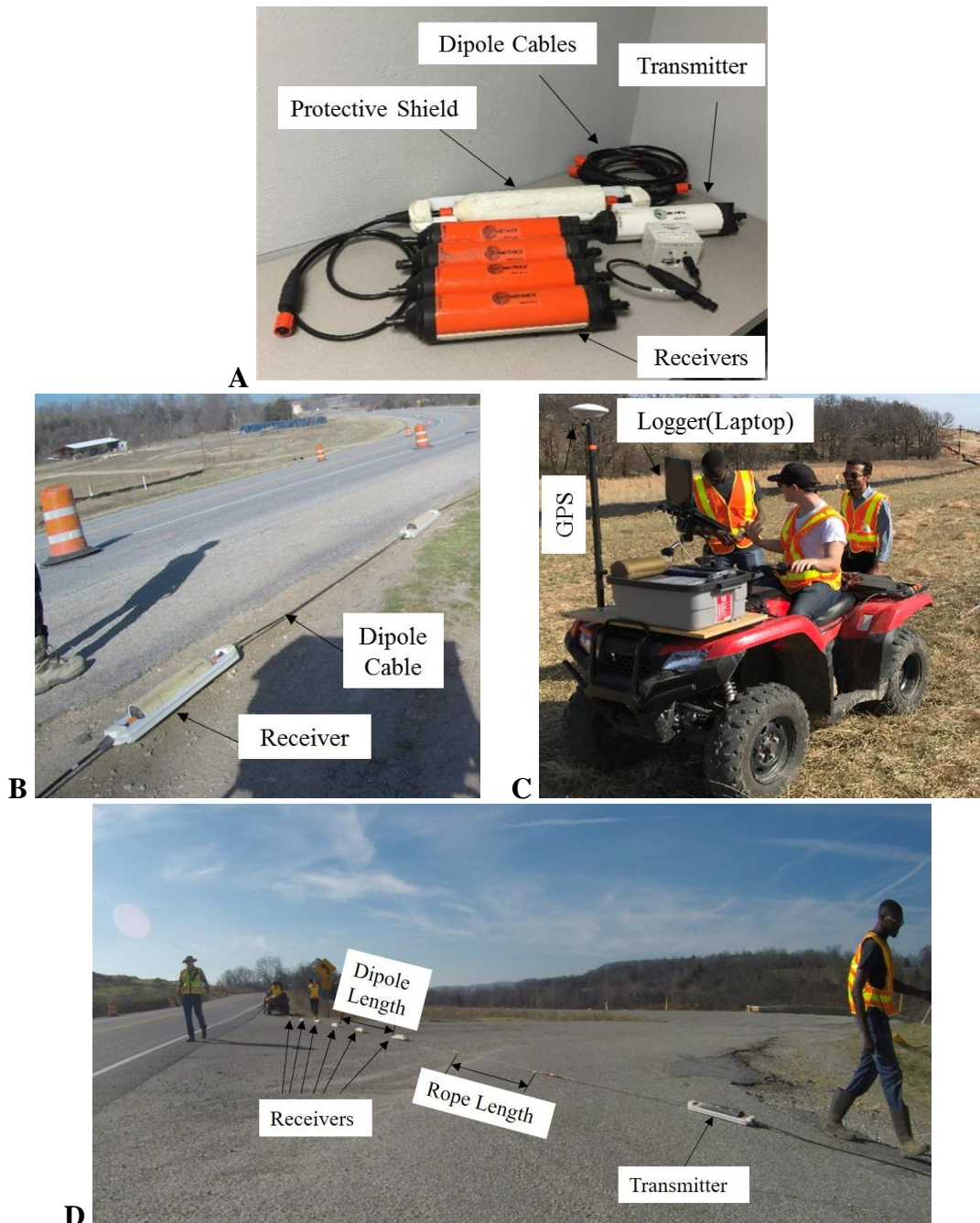
Figure 3-2. A) Transmitter and Receivers B) Dipole Cables connected to receivers with protective shields at the site. C) Data logger with Trimble Geo 7x GPS device mounted on the All-Terrain Vehicle (ATV) D) OhmMapper setup towed in a line by ATV along US 62 near Alpena, Arkansas.
